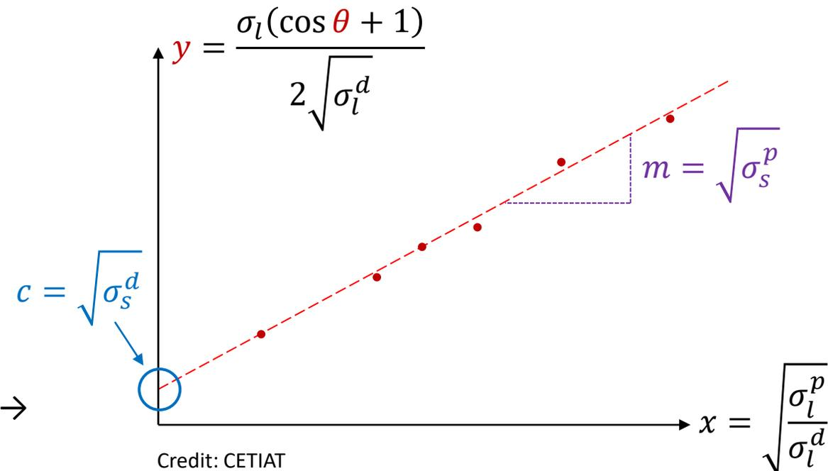
Several contact angle measurements with liquids of known surface tension may determine the surface energy of a sample  $\rightarrow$
