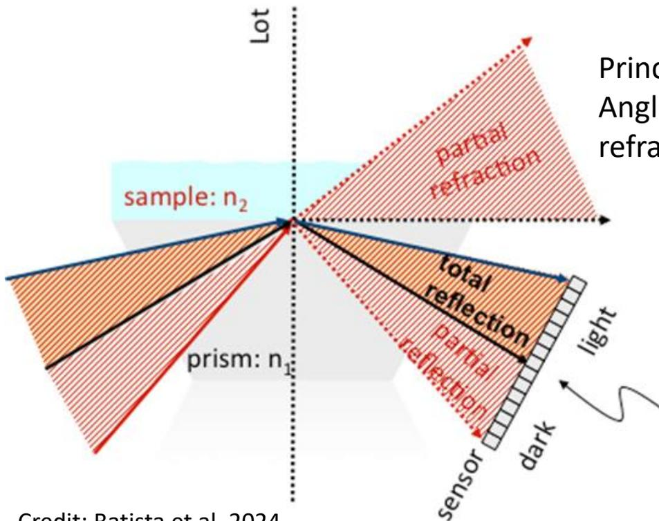
Principle of refractometer
