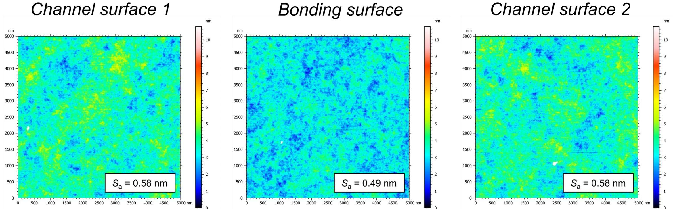
Channel surfaces were manufactured using wet etching, and appear more homogeneous than the bonding surface
