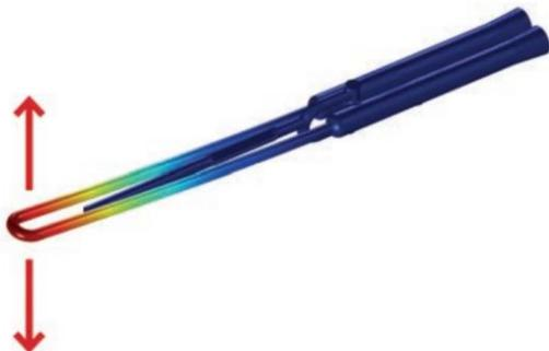
Some digital density meters use an oscillating U-shaped tube to determine density. The oscillation frequency depends on the density of the liquid filling the tube.
