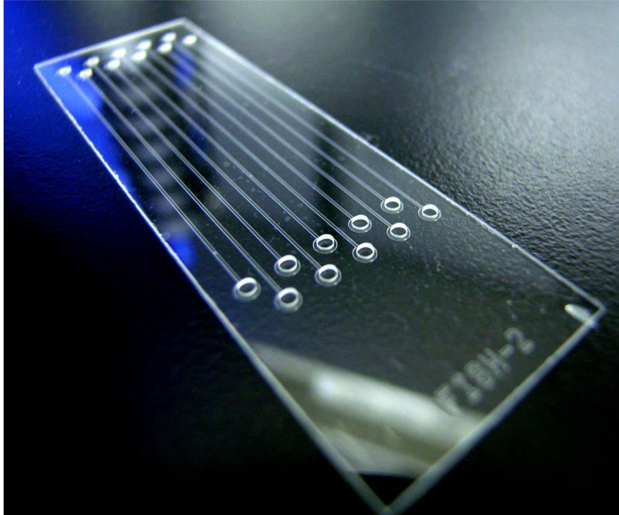
A microfluidic chip made of Polydimethylsiloxane (a polymer called PDMS) and mounted on a glass slide
