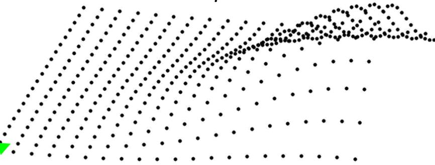
The instrument produces an image from the 3D point cloud acquired during the scan. Each pixel has XYZ coordinates, ideally acquired by position sensors.
