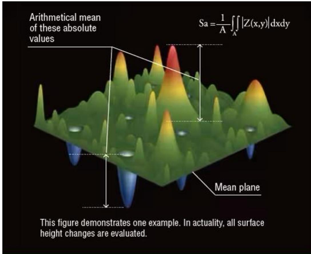
Surface roughness is quantified by surface roughness parameters, e.g. area surface roughness parameter  $S_a$
