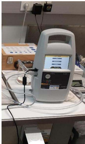
**Figure 5.** Infusion Device Analyser
