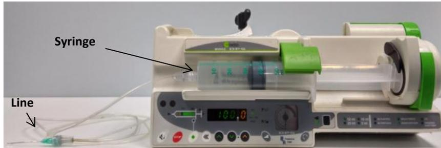
**Figure 3.** Syringe pump<sup>2</sup>
