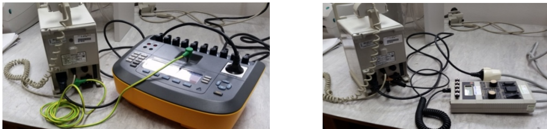
Figure 21 – Electrical security tests using a reference instrument
