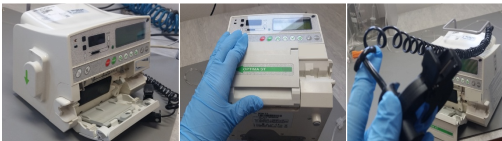
Figure 18: Visual inspection of a volumetric infusion pump: lateral verification (on the left); frontal (in the centre) and verification of the drop sensor (on the right).
