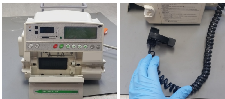
Figure 19: Visual inspection of a volumetric infusion pump: exterior and interior door (on the left) and drop cable sensor (on the right).
