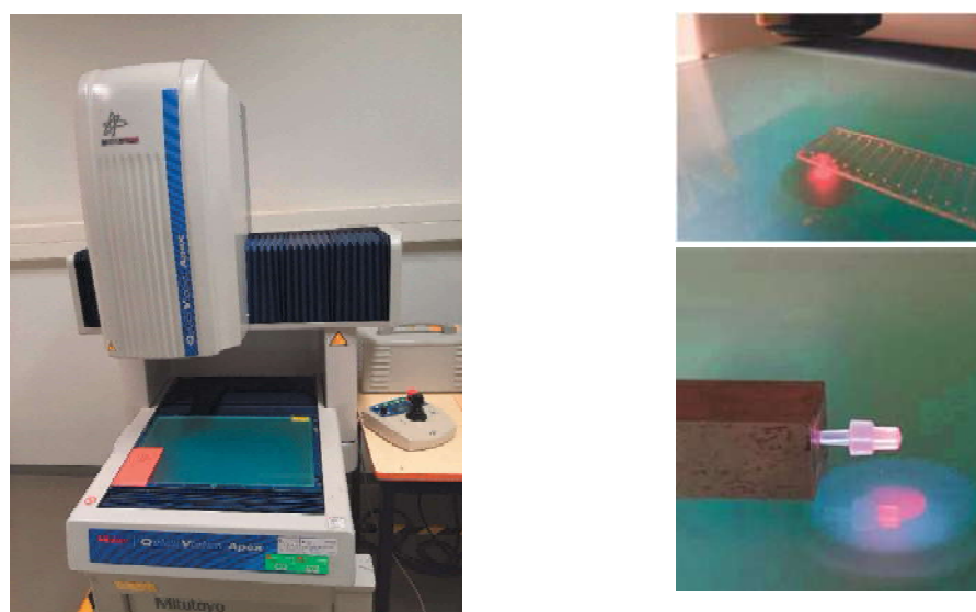
Figure 2. Three-dimensional optical measuring instrument and corresponding examples of use.
