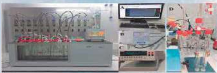
Figure 1 - Primary potentiometric system. A – Computer; B – Barometer, C – Multimeter and D – Harned Cell
