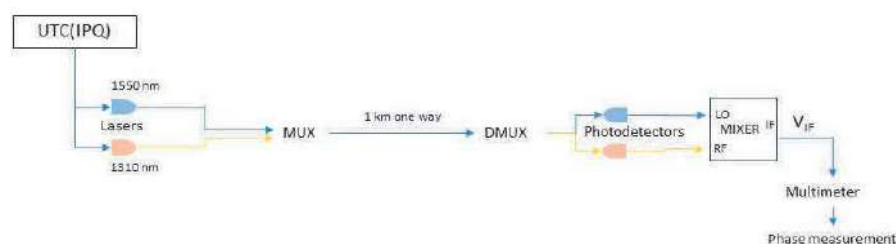
Figure 1. Representation of the physical system for phase measurement, which includes two lasers to transform the signal from UTC(IPQ) into light, two wavelength multiplexers (MUX and DMUX), two photodetectors to detect light, a frequency mixer, and a multimeter to measure voltage.
